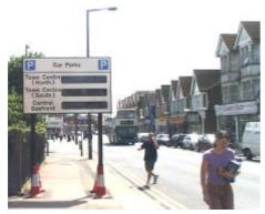
Variable Message Signs - will provide for the efficient management of traffic seeking available car parking spaces
