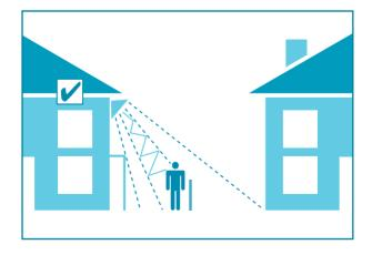
To reduce the effects of glare main beam angles of all lights should be below 70 degrees.
