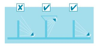
Do not install equipment which spreads light above the horizontal.
