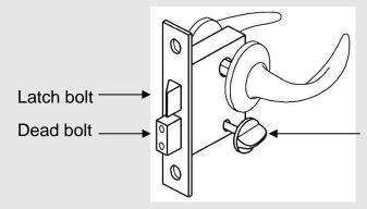
Note. The 'thumb-turn' operated lock should be sited on the room side of the door to facilitate escape without the use of a key.
