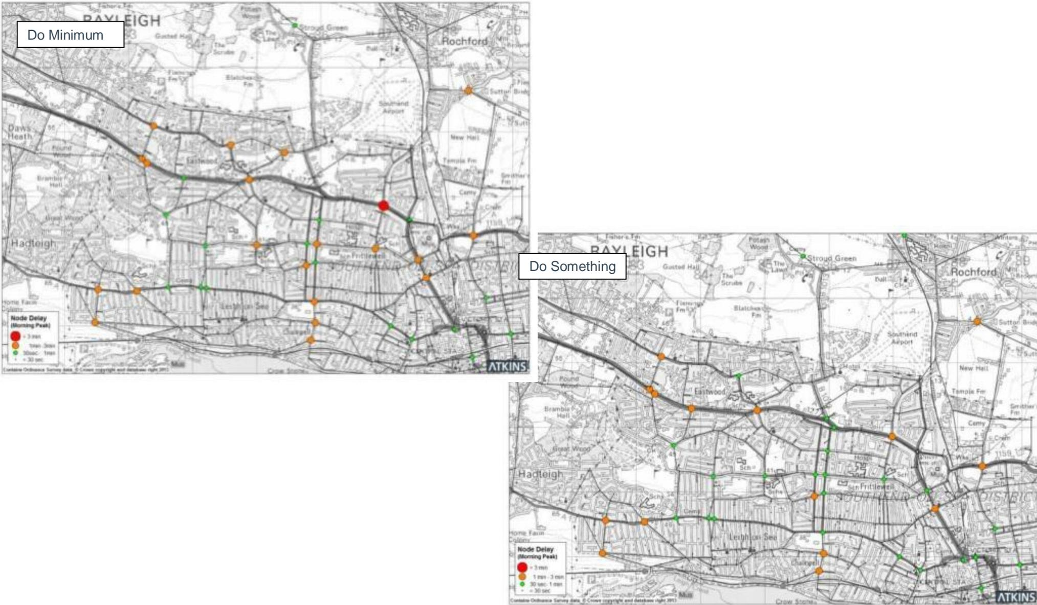
Figure 13. Highway Junction Delays Comparison PM Peak 2021
