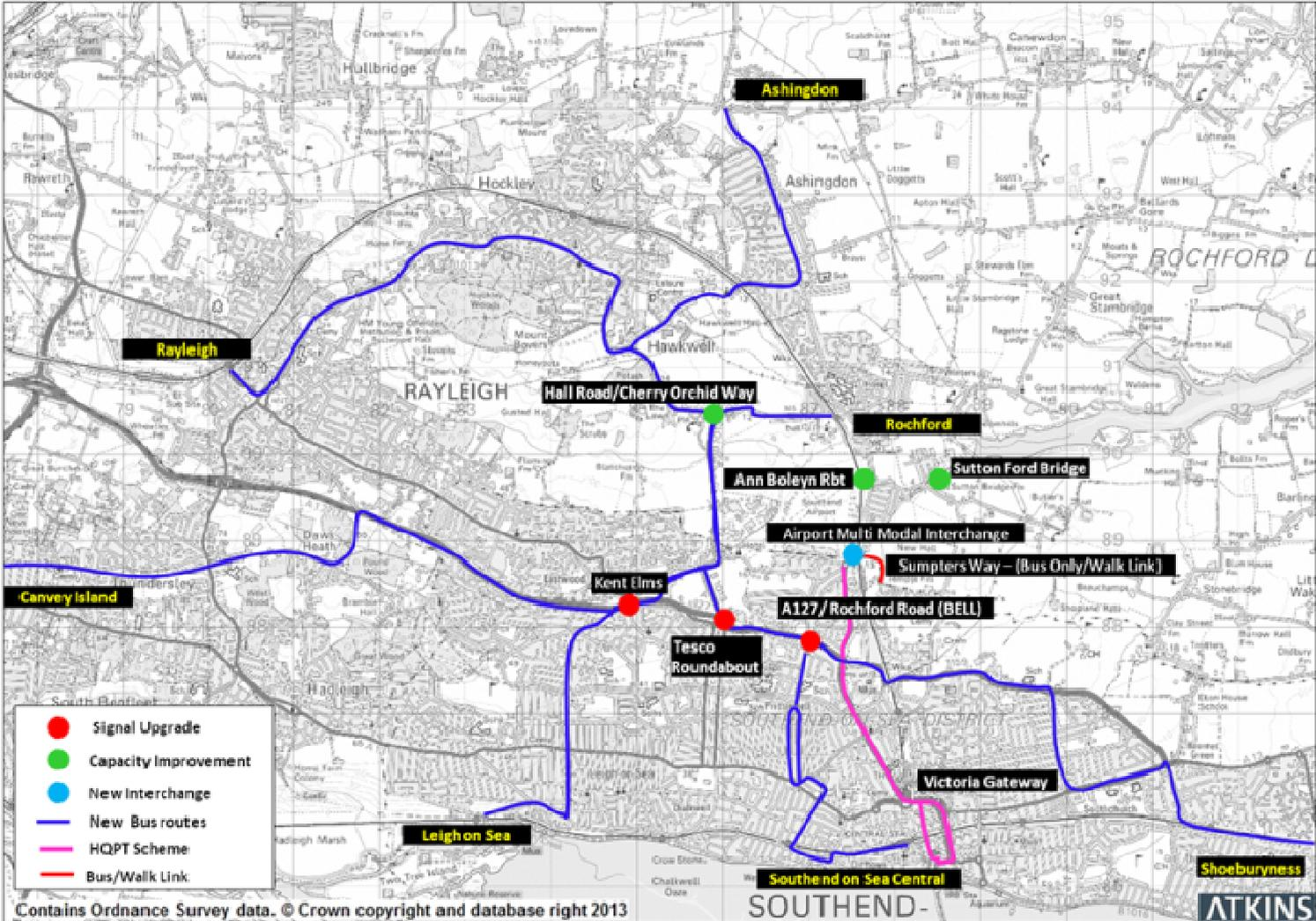
Figure 6. Junction Improvements - Existing vs Proposed
