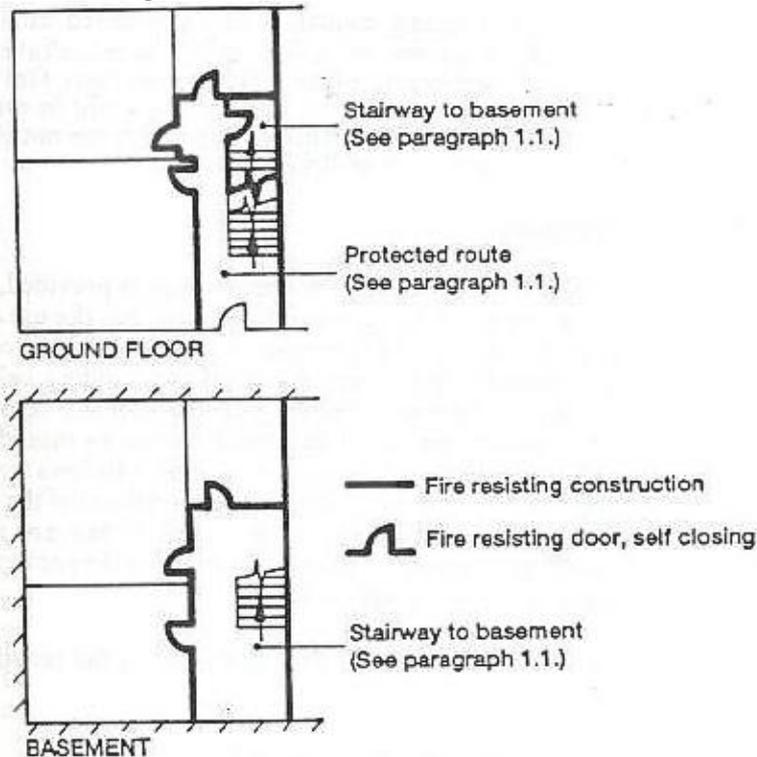
The basement is separated from the ground floor by 2 x 30 minute *fire doors*, one between any self-contained unit within the basement and one at the head of the stairway at ground floor.
