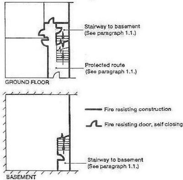
The basement is separated from the ground floor by 2 x 30 minute *fire doors*, one at the foot of the stairway and one at its head.
